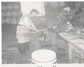
Cooper Elias Rafuse hammering a hoop at the W. G. Haverstock Cooper Shop in 1967
